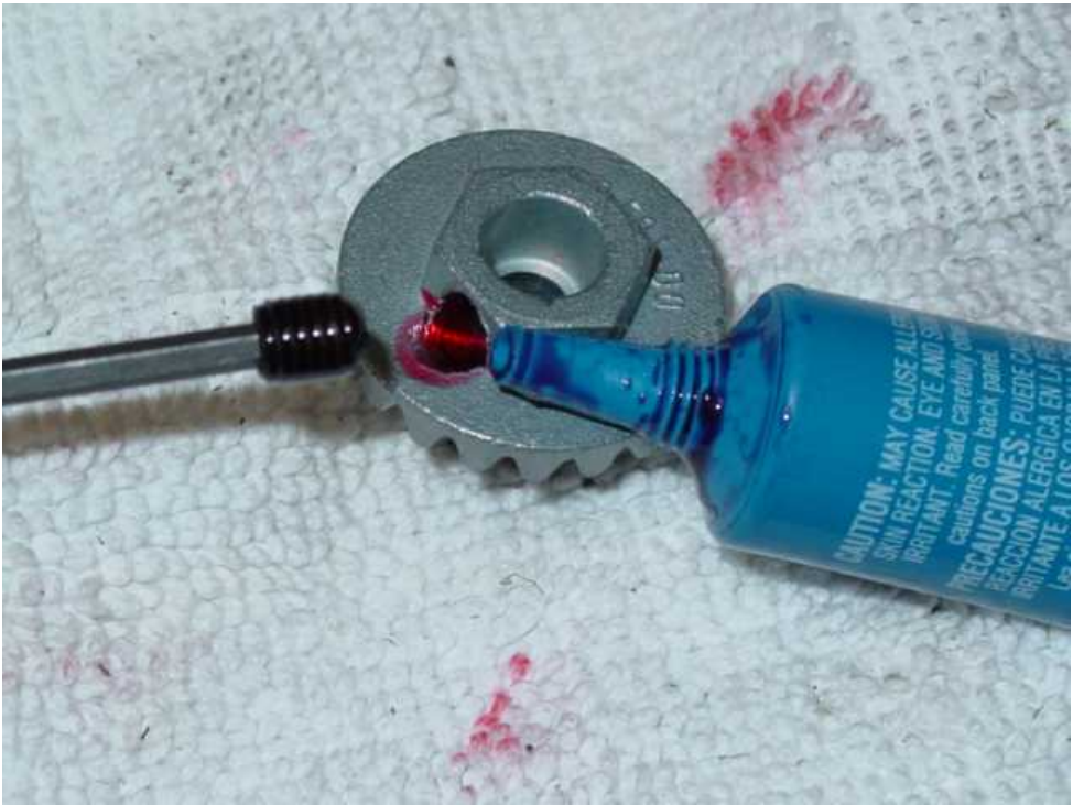
Be sure to use the suggested thread lock on the set screw.
