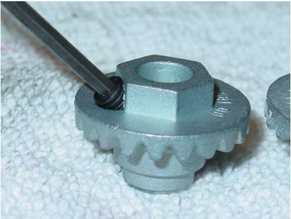
Be sure to use the suggested thread lock on the set screw.
